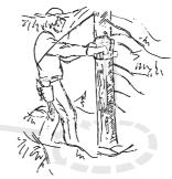
Remove any undergrowth from the base of the tree and check the area for obstacles (stones, branches, holes, etc.) so that you have a clear path of retreat when the tree starts to fall. Your path of retreat should be roughly 135 degrees away from the intended felling direction.
